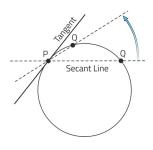
2. A measurement of slope at an instant. If f(t) is your distance at a particular time, its derivative, f'(t) is the rate of change, or the speed. It is equal to a tangent line at that point.
