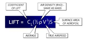
Increasing the density on the right hand side will increase the value of lift on the left hand side.
