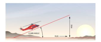
The horizontal distance is the *run*, and the change in height as you go along it is the *rise*. The ratio of the two is the degree of slope, expressed as a percentage when it comes to the climb. It is usually denoted by the letter *m*.
