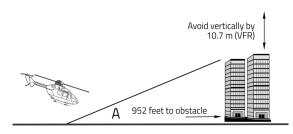
You first need to find the angle between the surface and the top of the obstacle. Angle A is 40°.
