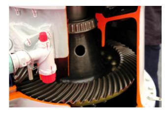
As contact between them is constant, smoother action is possible. As they tend to push each other apart, this action can be used as the basis of measuring the torque applied to a gearbox.
