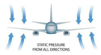
That is, the aircraft is being squeezed from all directions at a static pressure of around 2000 lbs per square foot. If you can reduce the pressure above its aerofoils by more than the weight of the aircraft, it will fly, which is what we do mechanically, by moving forward to concentrate the airflow over the top of the wing and bring its streamlines closer together.
