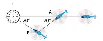
For example, it will take the same time to fly from point B in the picture to the navigation beacon as it does from A to B. It is a handy way of estimating time without taking you too far out of your way.
