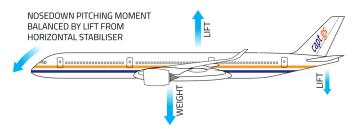
The size of a moment arises from the force involved multiplied by the distance from the point concerned to the line of action of the force. In the picture above, the two lift values are different, yet they
